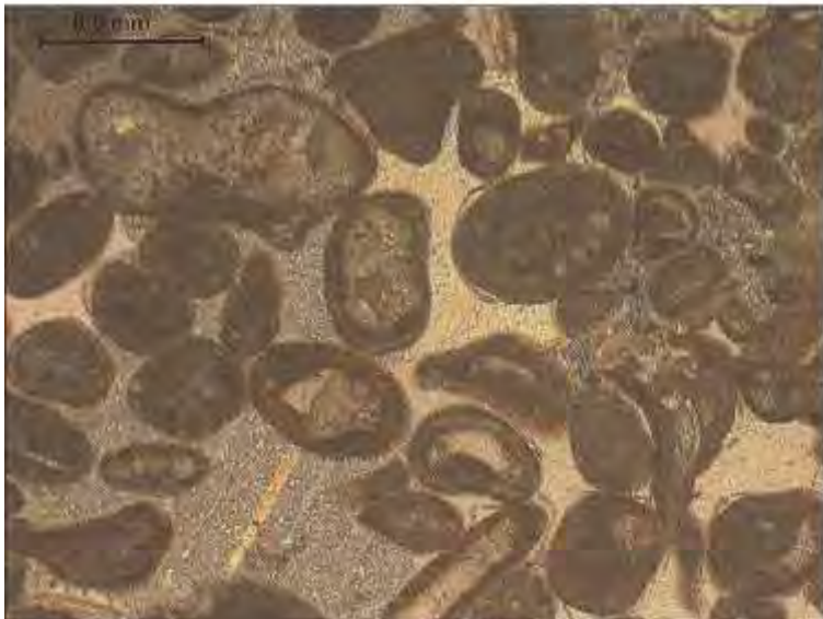
Figure 47 a-c: Roker Dolomite oolitic limestone: a) used as a building stone at St. Peter's, Wearmouth; b) photomicrograph showing the Oolite texture (ordinary light); c) photomicrograph showing the Oolite texture (polarised light).
