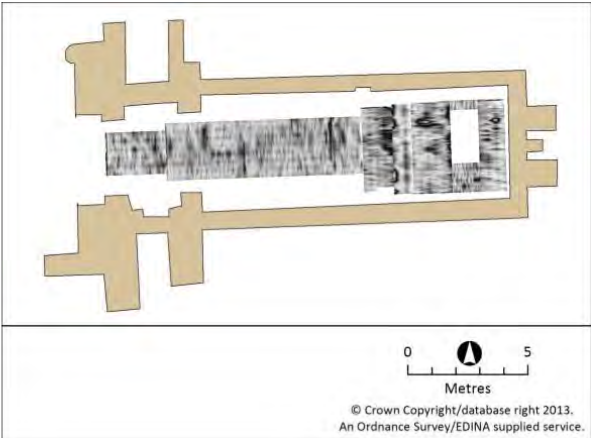
Figure 95: Internal GPR survey St Paul's Church, Jarrow, 2010. Plot at c.325cm
