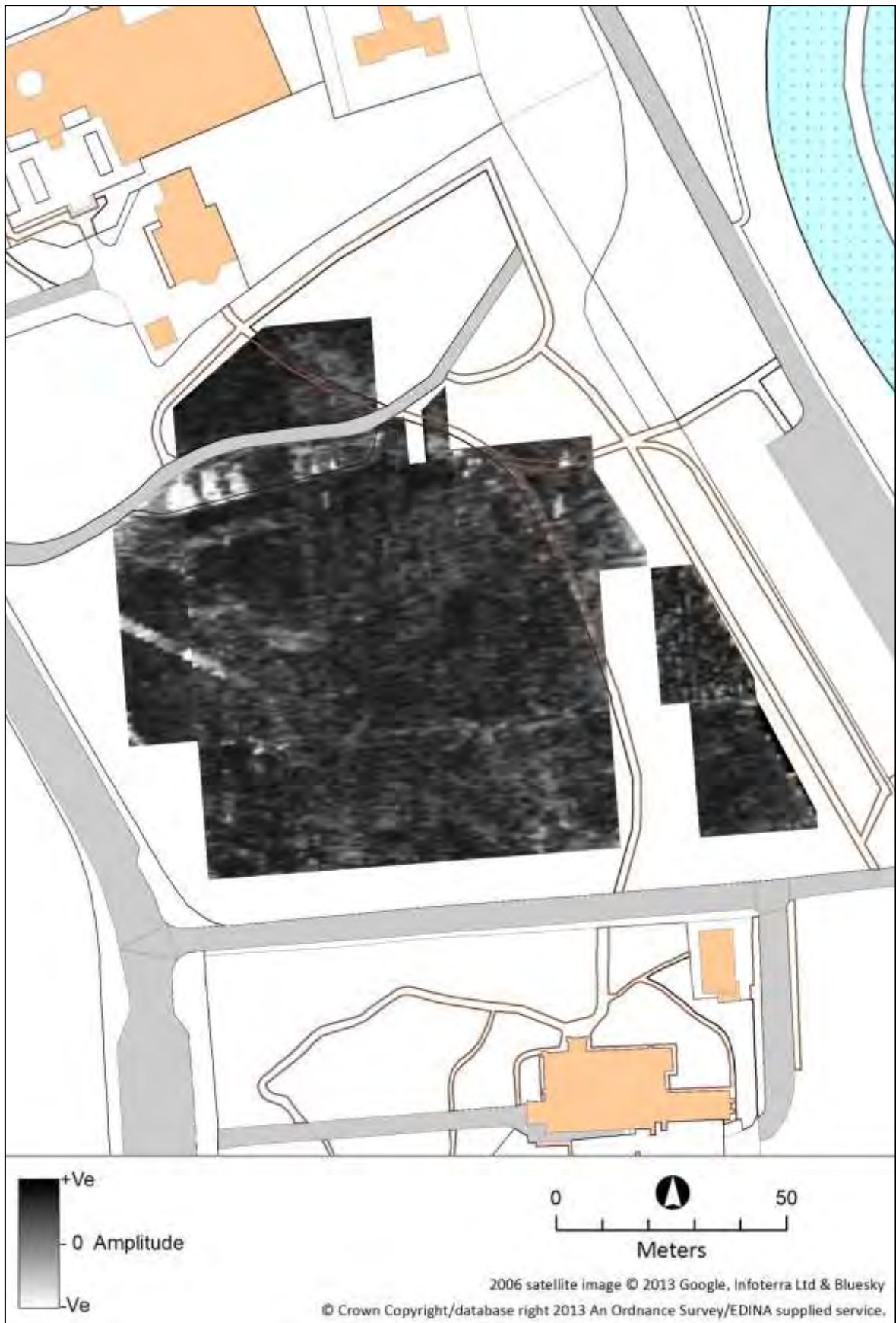
Figure 45: GPR results Drewett's Park, 2008 – depth c. 2.0 metres
