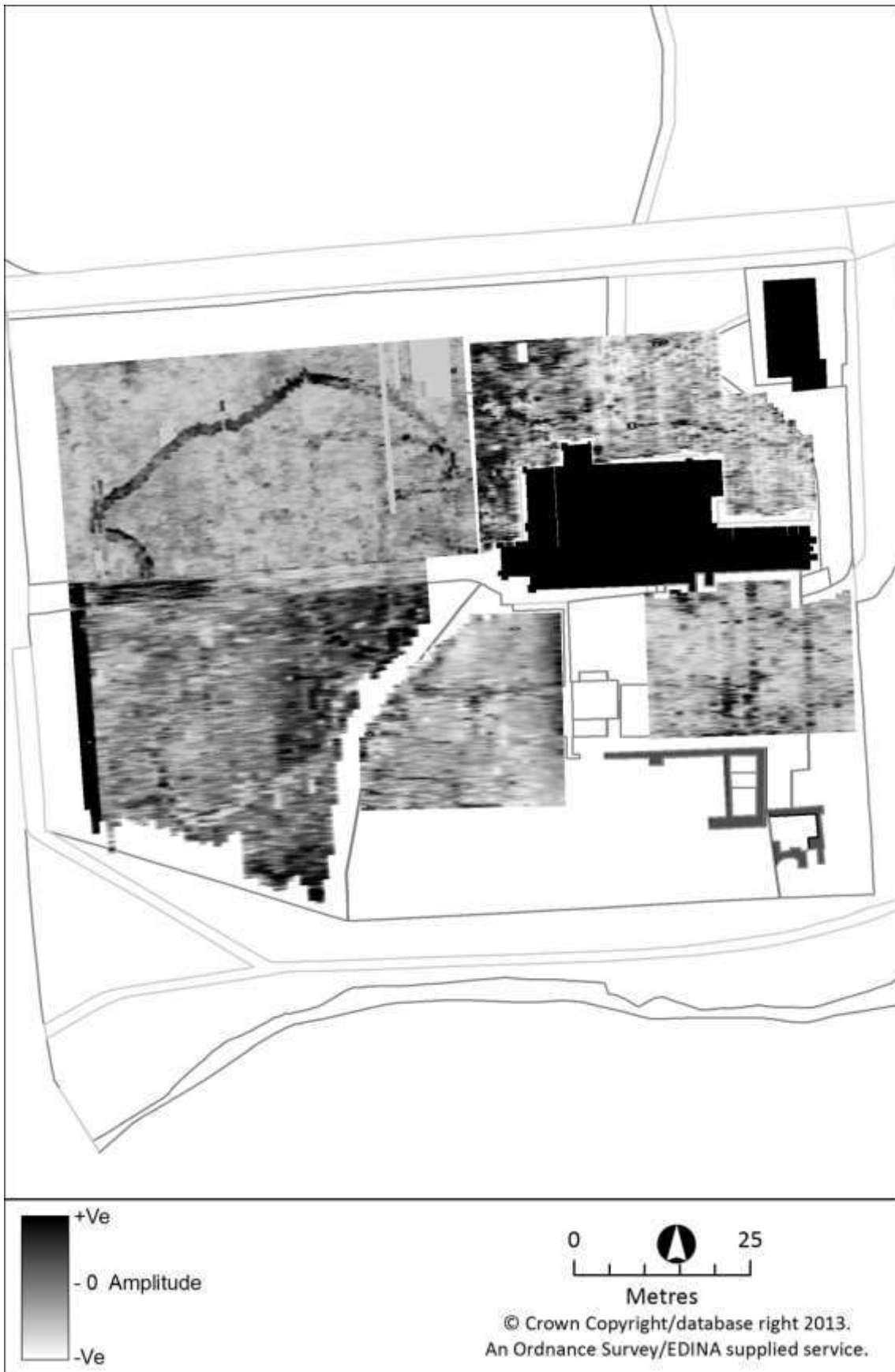
Figure 67: GPR survey results, St Paul's Church, Jarrow, 2009 – depth c.100cm
