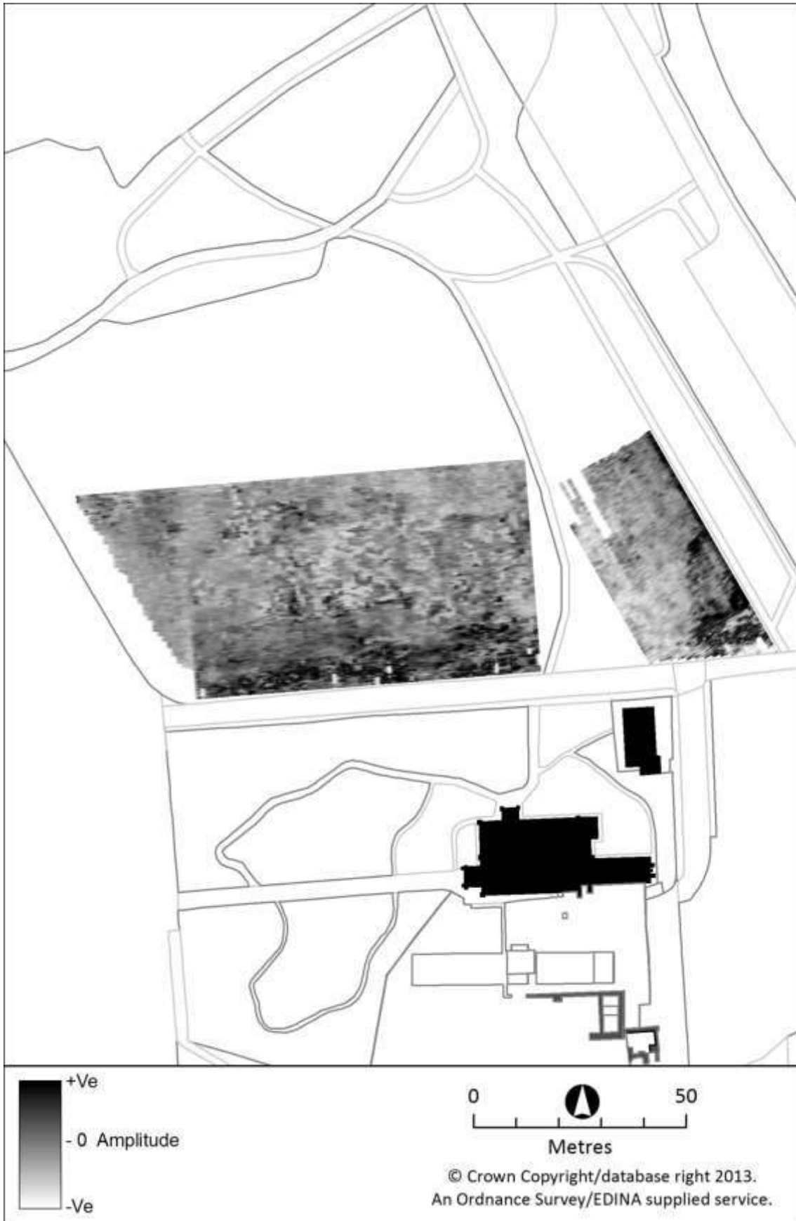
Figure 55: GPR results Drewett's Park, 2009 – depth c.1.25 metres
