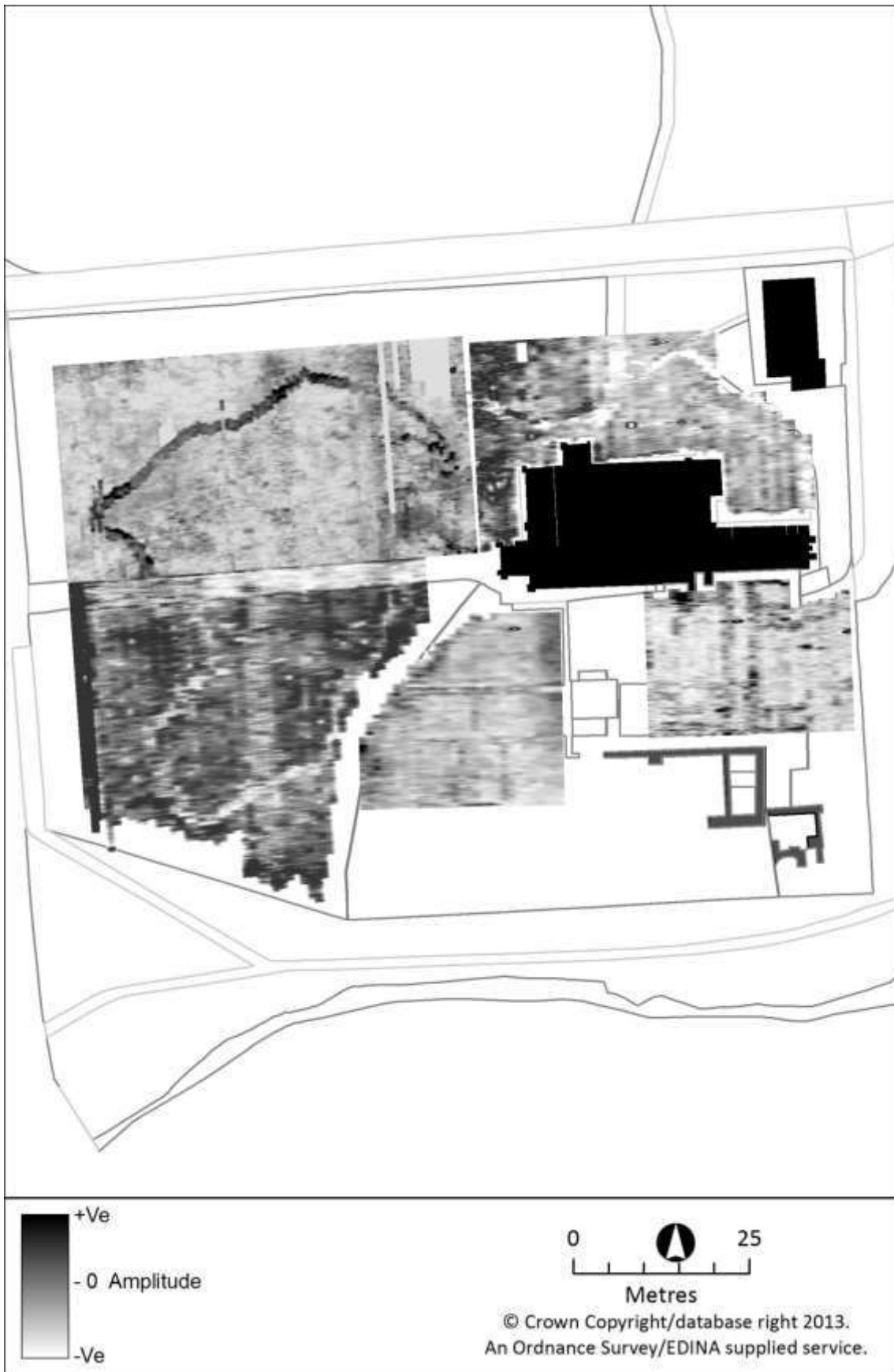
Figure 68: GPR survey results, St Paul's Church, Jarrow, 2009 – depth c.125cm
