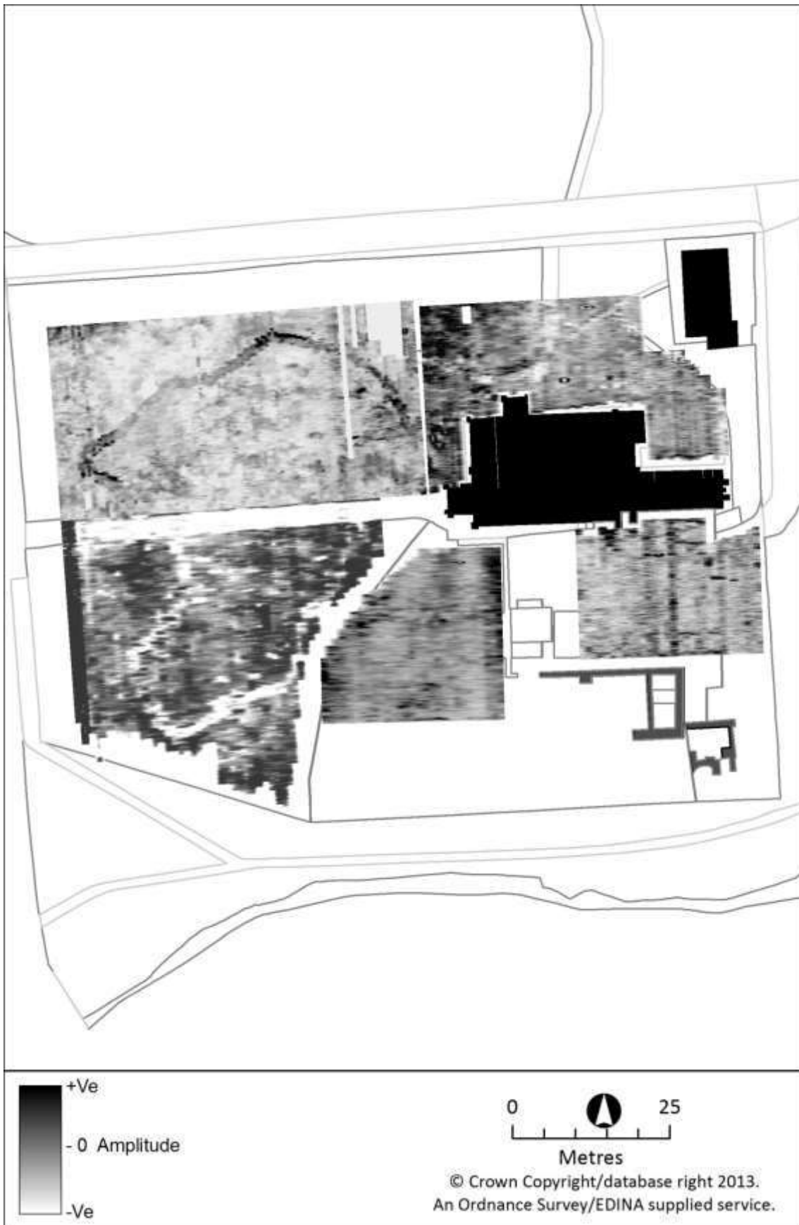
Figure 69: GPR survey results, St Paul's Church, Jarrow, 2009 – depth c.150cm
