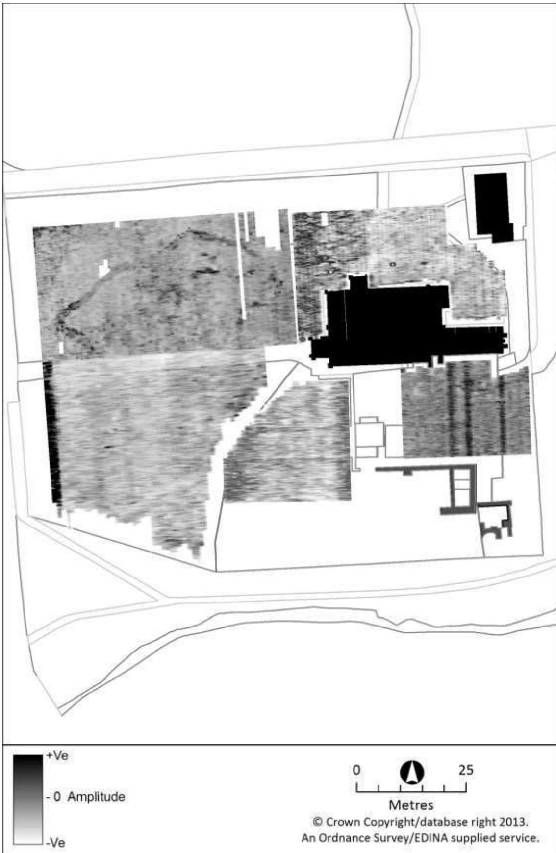
Figure 72: GPR survey results, St Paul's Church, Jarrow, 2009 – depth c.250cm
