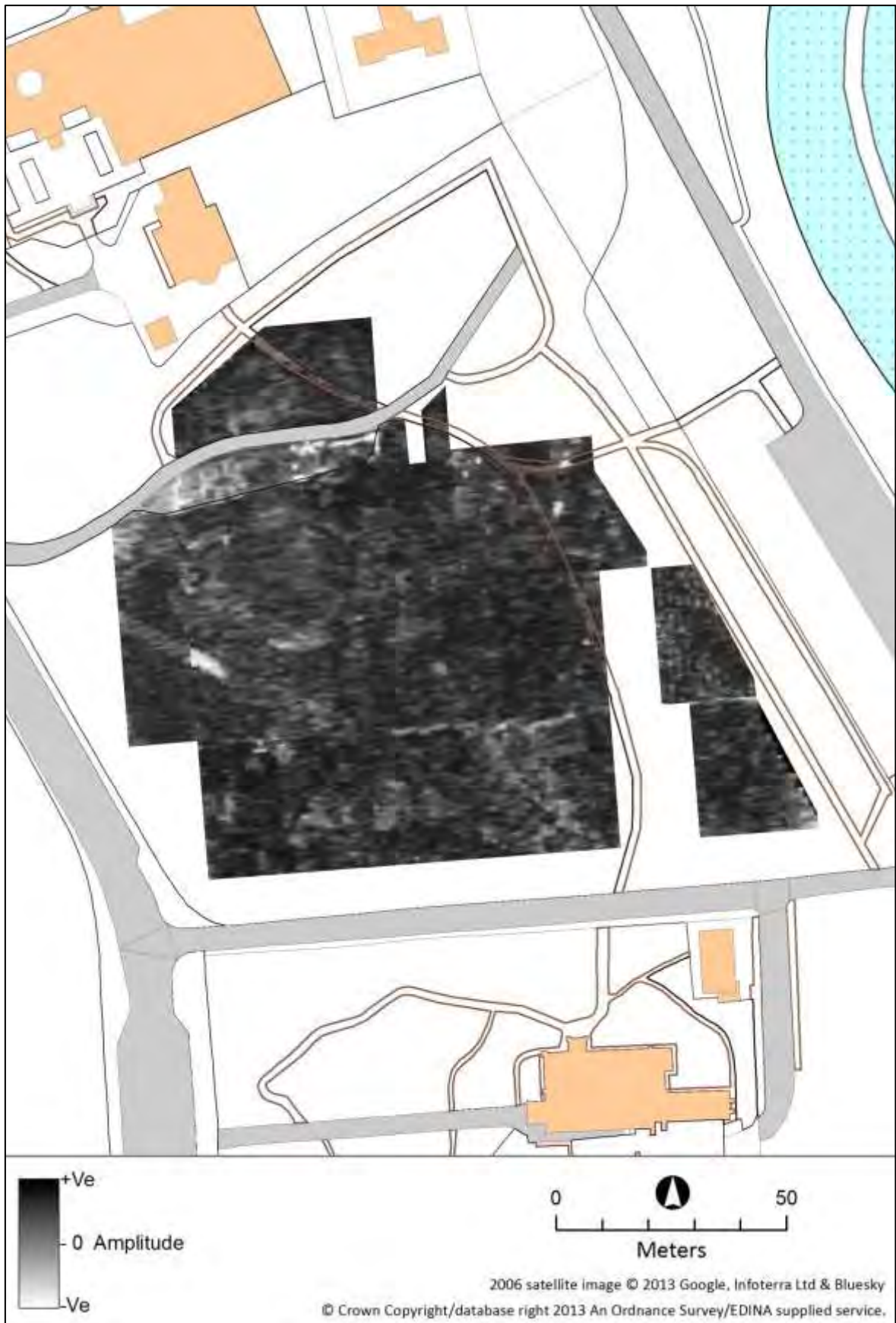
Figure 47: Figure 46: GPR results Drewett's Park, 2008 – depth c. 2.5 metres
