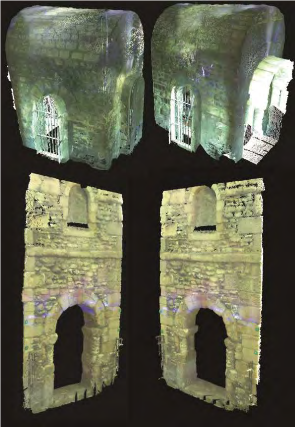
Figure 9: Internal (Top) and External (Bottom) point clouds for porch at St Peter's, Wearmouth viewed from west end. Opaque views using colours from camera.
