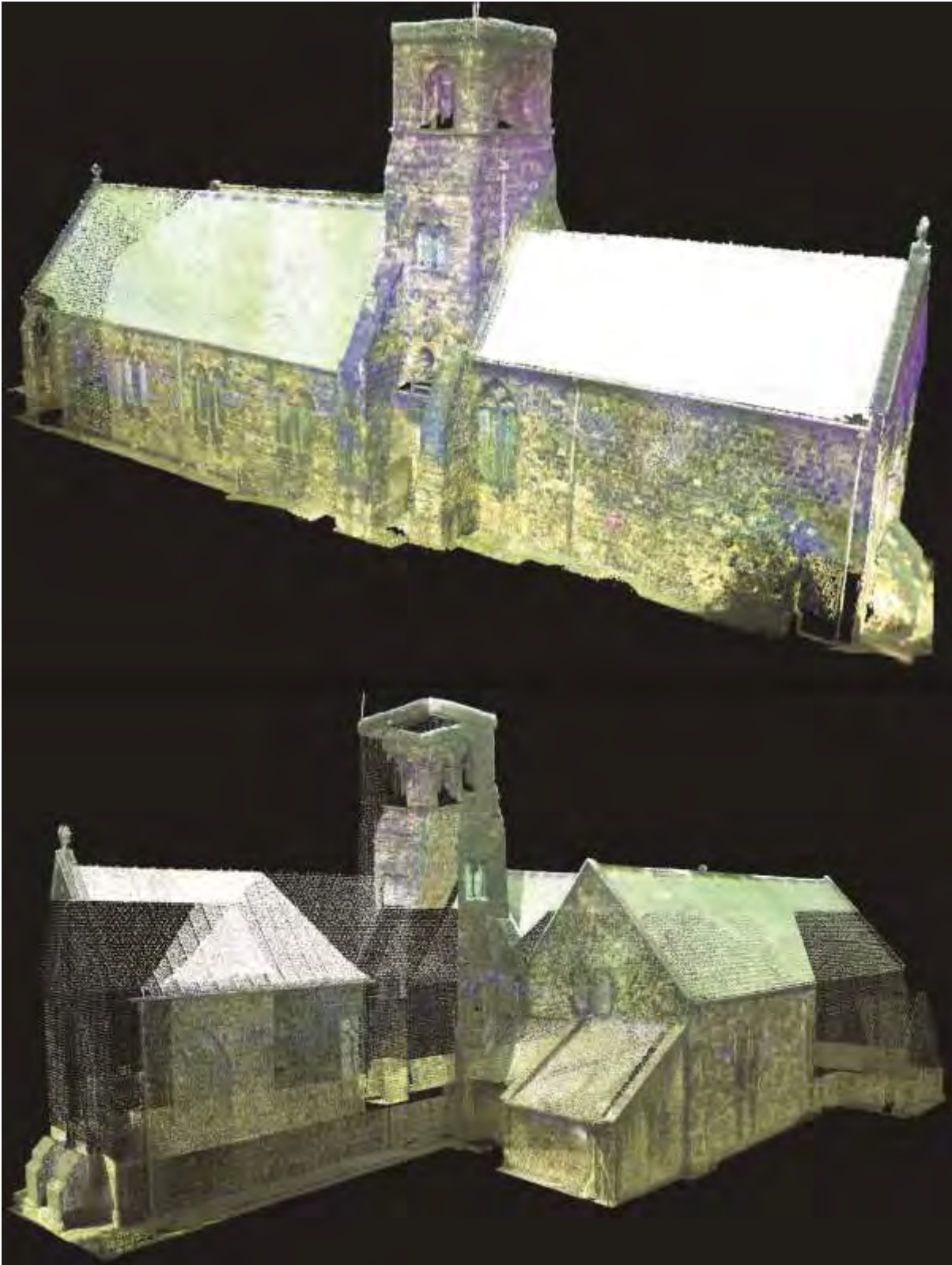
Figure 5: Point cloud for St Paul's, Jarrow viewed from east end. Top opaque view and bottom transparent view using colours from camera.
